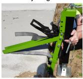
**Step 2.** Place lifting frame into place and lifting jack behind it.
