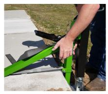
**Step 6.**Pull extra strap tight and ratchet strap firm so that frame is tight against concrete.
