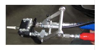
**8.** Attach Equalizer to A (red) and B (blue) heated hose and flush line. Use two wrenches and be careful not to overtighten.
