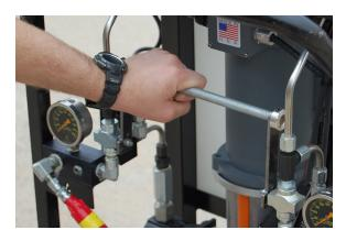
**1.** Re-circulate until material has reached factory recommended temperature.
