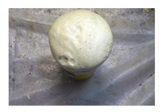
**8.** Review material for cream, gel, and rise times. Properly reacted material produces a smooth, hard foam. Crunch foam is usually A-rich. Spongy foam is usually B-rich.
