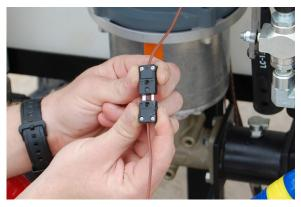
**3.** Connect thermocouple wire to hose with minipin connected; wrap with electrical tape to avoid false readings.
