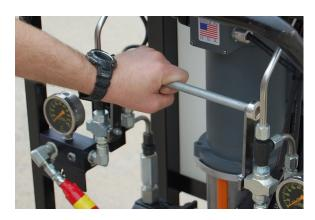
**7.** Return actuation handle on machine to re-circulate position (up).
