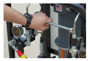
**7.** Shut machine off, return actuation handle to vertical (up, re-circulate) position.
