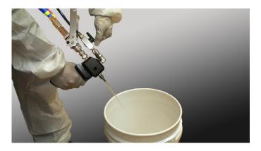
**6.** Pull Equalizer handle back to rear position and flush with three quick bursts of water away from the reacting material or in another pail or bag; engage safety knob.
