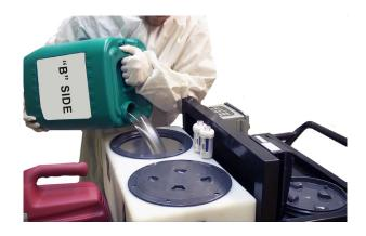
**1.** Pour desired amount of material into each tank. Again, only open one tank at a time to avoid cross contamination.
