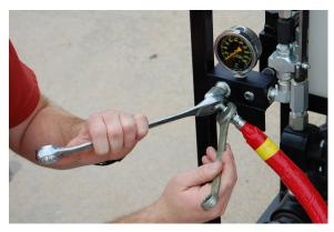
**5.** Tighten hose connections at machine, using wrench. Do not over tighten, JIC fittings do not require Teflon tape or pipe dope. Special care should be given to not twist hose, 2 wrenches are required.
