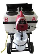
**6.** Prepare flush by installing pump on rear carriage, (locking tabs on frame) and inserting dip tube into flush bucket. Plug flush pump electrical cord into receptacle located on side of box. DO NOT POWER ON FLUSH PUMP. Connect flush hose to the 1/4" fitting on the left side of the flush pump.
