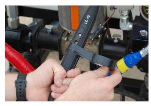
**4.** Plug heated hose together and twist to lock; ensure by attempting to pull apart. Once lugs are properly connected, tape joint to secure.
