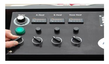
**2.** Turn motor switch to on position and slowly increase speed knob to 4 (ensure actuation handle is in up position, re-circulate).
