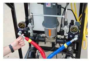
**2.** Attach hose to corresponding fitting on Revolution machine, A-#5 JIC, B- #6 JIC and tighten to finger tight only (to be further tightened later).
