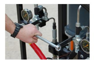
**4.** Engage actuation handle to dispense position (down) at machine. (The motor may bump a couple of times to achieve pressure.)
