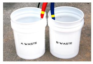
**2.** Place the ends of the A (red) and B (blue) heated hose in separate waste buckets.
