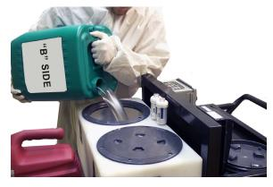
1. Put approximately  $\frac{1}{2}$  gallon of material into each tank, making sure A and B material go into corresponding A and B tanks. Remove only one lid at a time to prevent accidental drips into the other tank.
