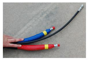
**1.** Identify A (red) and B (blue) heated hose ends. Lay hoses out flat and avoid kinking.
